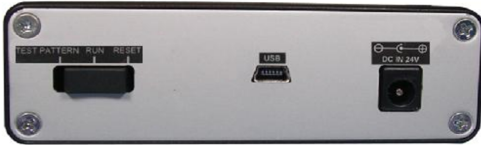
Figure 2.4.1 GRT SAM DC power connection and Toggle Switch
