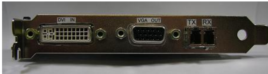
Figure 3.5 Gravity back plate with DVI input connector
